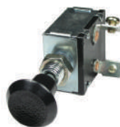
SPST Push-Pull Switch 12V @ 15A 1/2" Mount Hole On-Off
