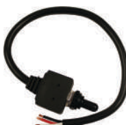
Weather Resistant Momentary SPDT Switch Controls two single wire circuits, permitting only one circuit to be energized at a time. Switch has a special rubber coated casing to resist moisture. Weather resistant boot included. 24V @ 15A / 12V @ 25A Mom On-Off-Mom On
