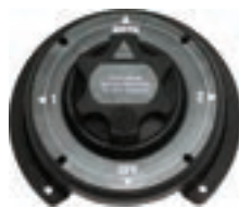
Marine I & II Dual Battery Selector Switch Master battery selector and disconnect switch for application up to 36VDC, 4 positions-both/1/off/2. Rating: 310 Amps Continuous 500Amps/5 mins.
