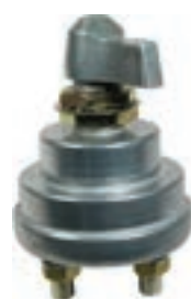
UL 588 Heavy Duty Master Battery Disconnect Disconnects battery circuit only. Does not disconnect alternator or generator field circuit. When used on alternator equipped vehicles, the engine should be stopped before switching to the OFF position to prevent possible alternator diode failure. 6-36V DC, 3/4" Mount Hole 190A Continuous, 1000A Momentary
