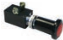
Illuminated SPST Push-Pull Switch 12V @ 15A / 6V @ 25A Bulb No. 282 1/2" Mount Hole On-Off
