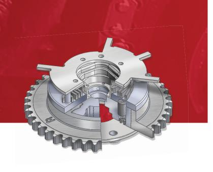
For 3V Ford 4.6-liter and 5.4-liter applications, Cloyes has developed a uniquely designed actuator that is superior to the OE product. Testing against the OE actuator, the Cloyes units exhibited 20% less frictional drag and produced 10% more torque at the same oil pressure. The Cloyes actuators use tightly toleranced, long duration rotor vanes that eliminate the wear and drag of the OE and other aftermarket designed units.
